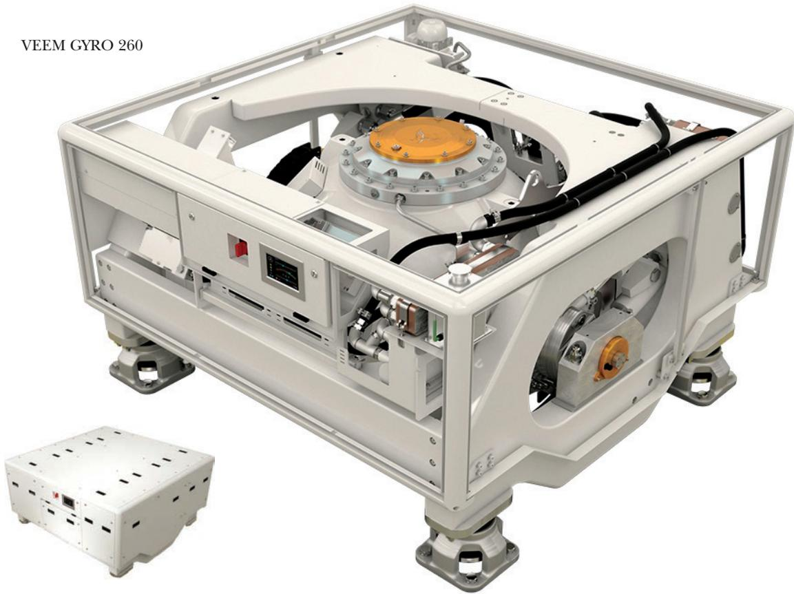
this dead-band. This option may be advantageous for some megayachts, or larger commercial vessels. The downside is the additional power requirements, space and cost of the motive power unit. The driven precession oscillation option requires either PTO hydraulic pumps or a separate power pack.
